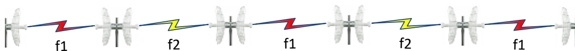
Figure 1 Data Pipeline showing the operation at alternating frequencies on every hop. The MagiNodes are connected back-to-back using their Ethernet ports.
